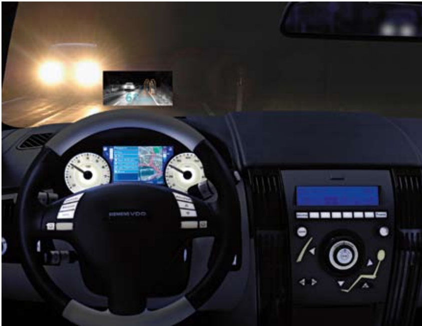
Fig. 4.5.11 A night vision system for pedestrian safety © Siemens
